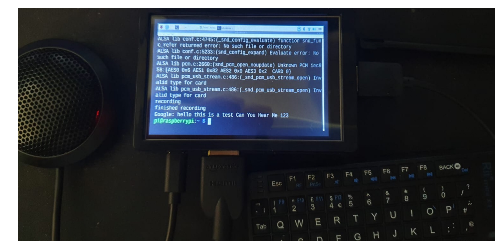
Figure 5 – Raspberry pi showing the transcription.
