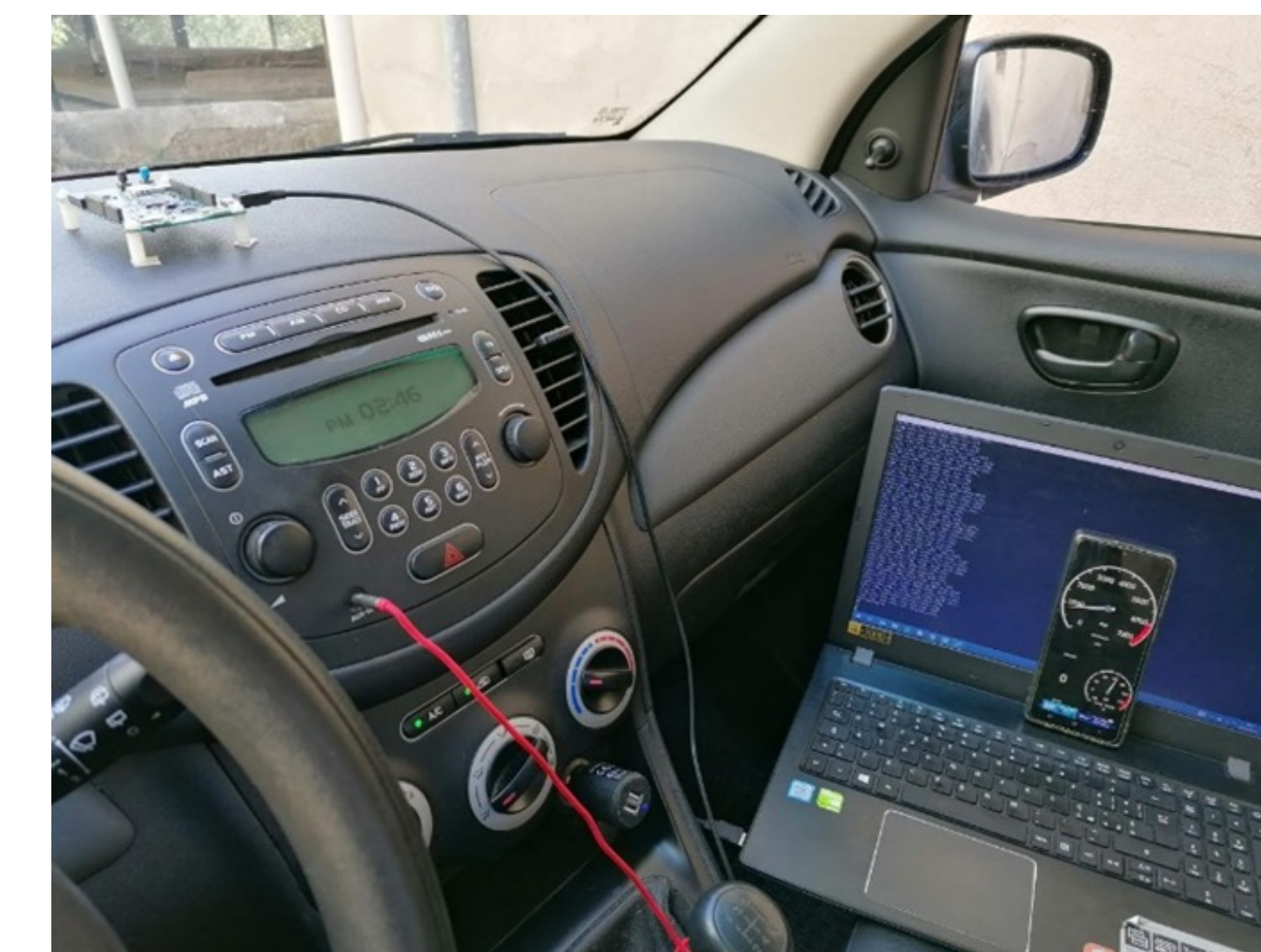
Figure 7: Setup used for onboard data acquisition to create datasets.
