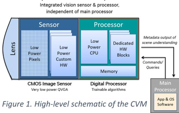
Figure 1. High-level schematic of the CVM
