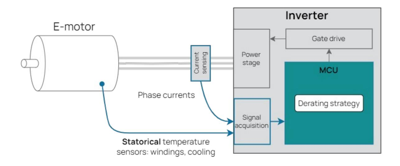
The motor control applies a derating strategy based on windings temperature
