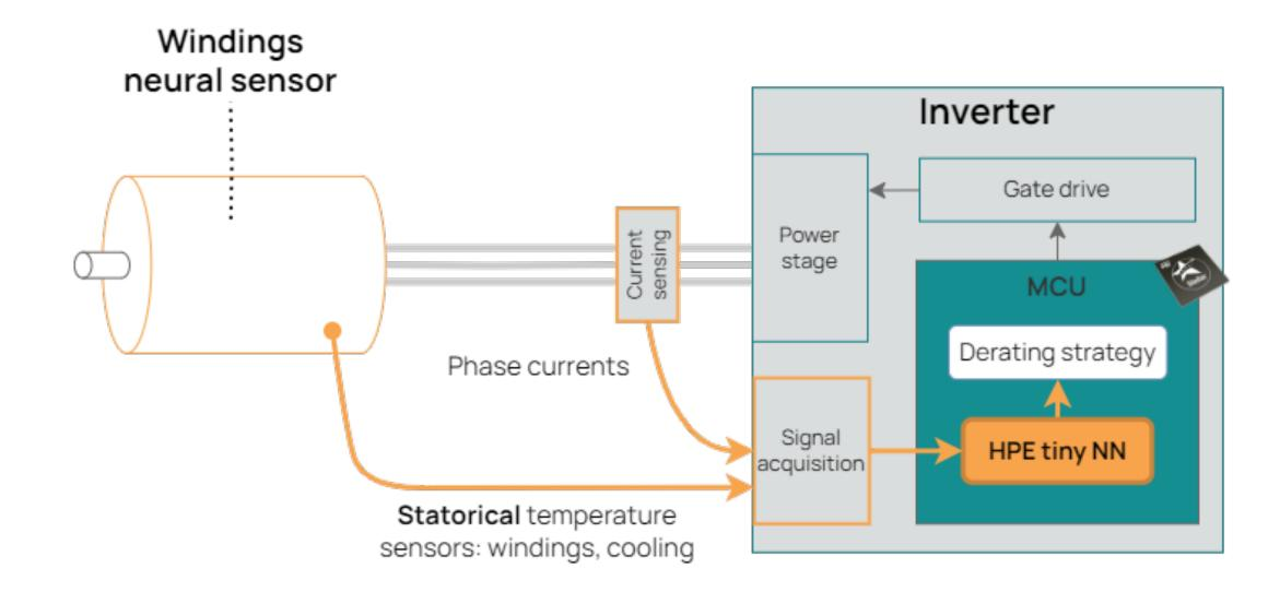
The HPE tiny NN also estimates windings temperatures to ensure continuous operations in case of real sensor failure
