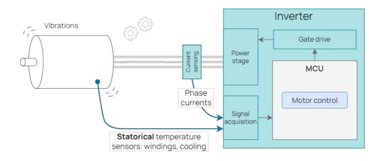
The standard practice is to implement over-current and over-temperature protection mechanism to address mechanical failures
