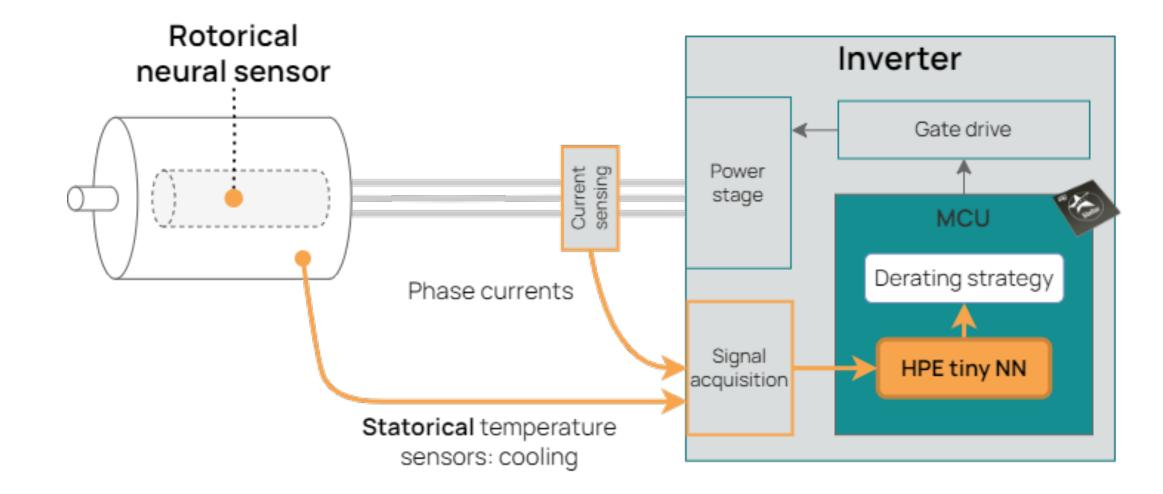
The HPE tiny NN virtualizes the magnets temperature sensor
