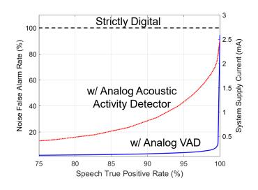
Low false-alarm rate is critical for low system power
