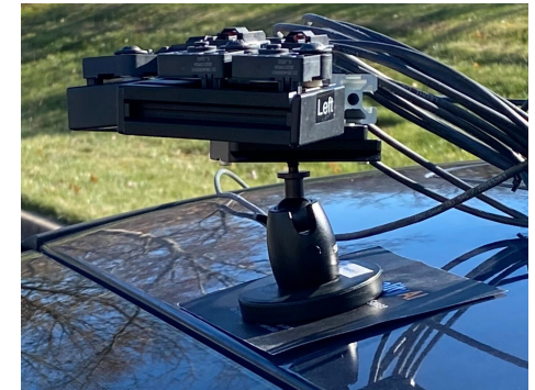
Prototype rooftop SWS array featuring automotive-grade mics from
