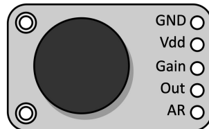
Electret microphone with MAX9814
