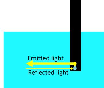
Light is reflected by particles in the liquid -> More reflected light = higher turbidity
